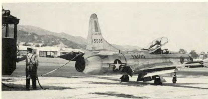
After sliding 2500 feet with its main gears cocked at a 90-degree angle, this F-94C came to a stop with two tires blown. Landing was possible because of 3500 feet of foamite spread on runway.
