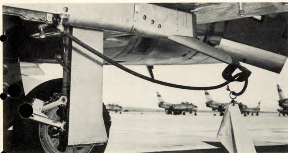
The attaching leader is passed through the guide and the release ring is hooked into the shackle. The aft end of the leader is temporarily wired around the guide, until tow cable hookup is made.
