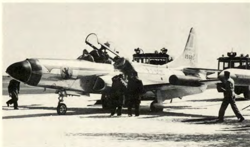
After sliding 2500 feet with its main gears cocked at a 90-degree angle, this F-94C came to a stop with two tires blown. Landing was possible because of 3500 feet of foamite spread on runway.
